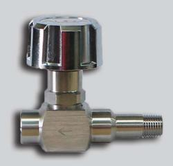
The AURA EXPVD Series diaphragm valve provides primary flow control in high-purity or corrosive gas systems. The packless, springless design enables compatibility in high-purity systems and extended lifecycle, while the Elgiloy diaphragm increases accuracy and repeatability even under harsh process conditions. The configurable inlet and outlets allow for easy installation and drop in replacement.
